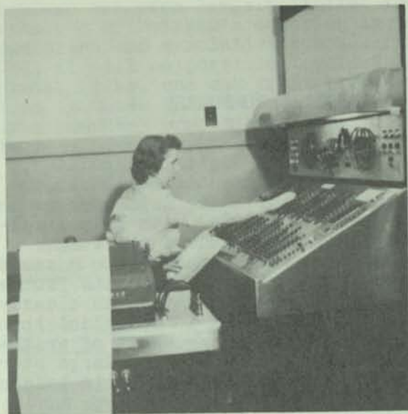
Figure 6—Operator Preparing Input Tape for ADEC.
